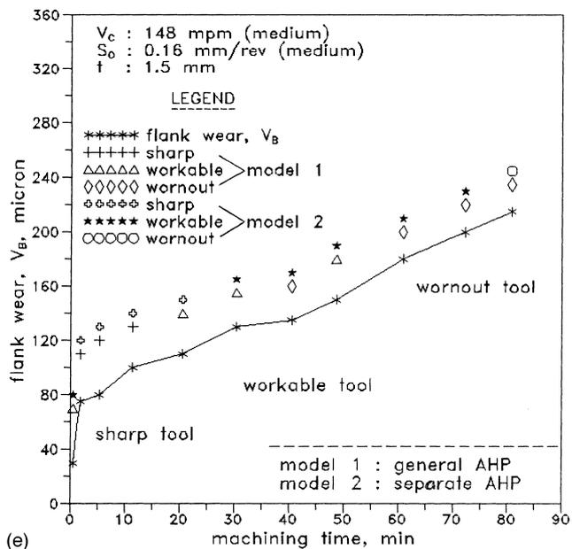
**Fig. 3** Predictability of the tool condition by the AHP under (a) low speed and low feed machining, (b) high speed and low feed machining, (c) low speed and high feed machining, (d) high speed and high feed machining and (e) medium speed and medium feed machining
