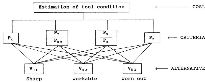
**Fig. 1** Hierarchy of the tool condition monitoring system
