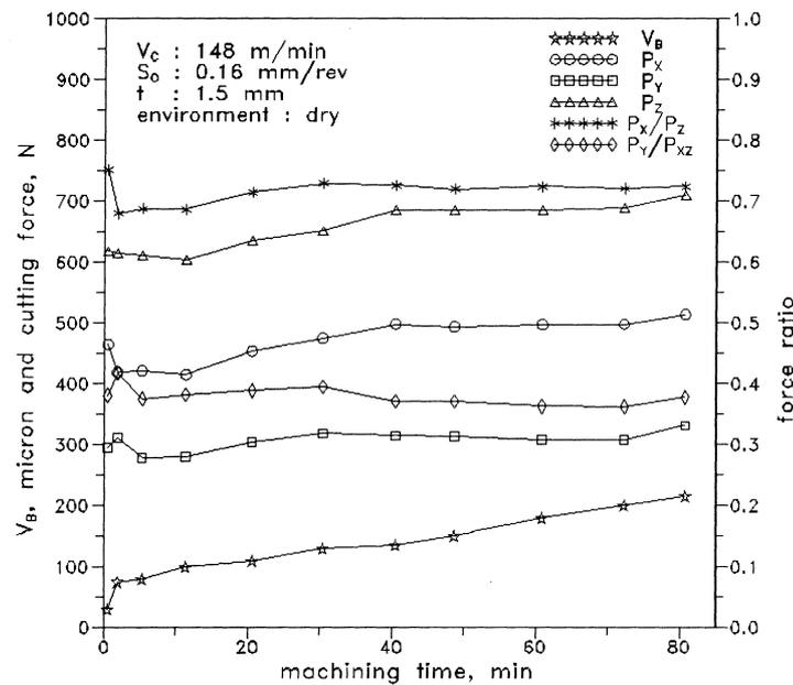
**Fig. 2** Growth of flank wear and increase in cutting forces with machining time at the medium speed–feed condition
